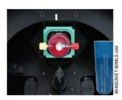
Push the 'Lock' button on control panel and open the upper lid. Place APS Separator into centrifuge. Be sure the centrifuge is balanced with a counterbalance or a second full APS Separator.
