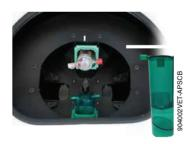
Place the Pro-Stride device into the centrifuge. Balance centrifuge with Pro-Stride/APS counterbalance or a second full APS concentrator. Spin for 2 minutes at 2000 RPM.
