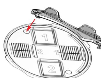
Place the Key on the assembly so that the two knobs on the underside of the Key fit into the two holes on the Reading disc.
