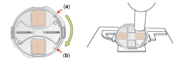
After 10 minutes, the Key is used to turn the reading disc clockwise (about 90°) until the Reading disc stops moving from (a) to (b). Remove the key. Attach the Microscope adaptor to the microscope and place the Mini-FLOTAC on the Microscope adaptor with the ruled grid No. 1 on the right.
