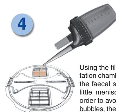
Using the filling holes, the flotation chambers are filled with the faecal suspension until a little meniscus is formed. In order to avoid formation of air bubbles, the chambers should be filled with the Mini-FLOTAC apparatus held at a slope.
