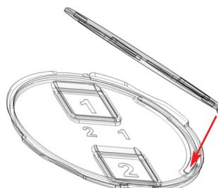
Place the lower side of the Reading disc onto the upper side of the Base, so that the small knob of the Reading disc enters the base slot.
